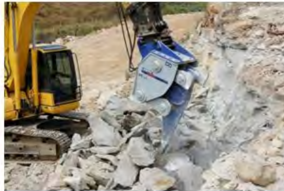
"XR20" is attached to a Komatsu hydraulic excavator.
