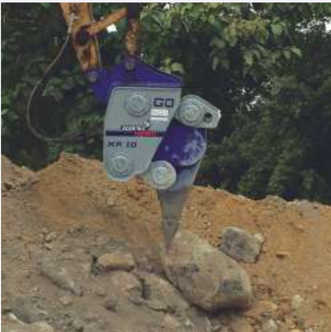
XR10 on the CAT Excavator working at the local Cement factory breaking up Clinker in a shed and outside.
