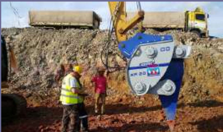
Checking the hydraulic pressure in the return line of XR20.
