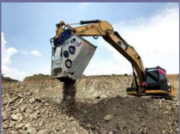
XC20 crushing rock at maximum output of 150 mm.
