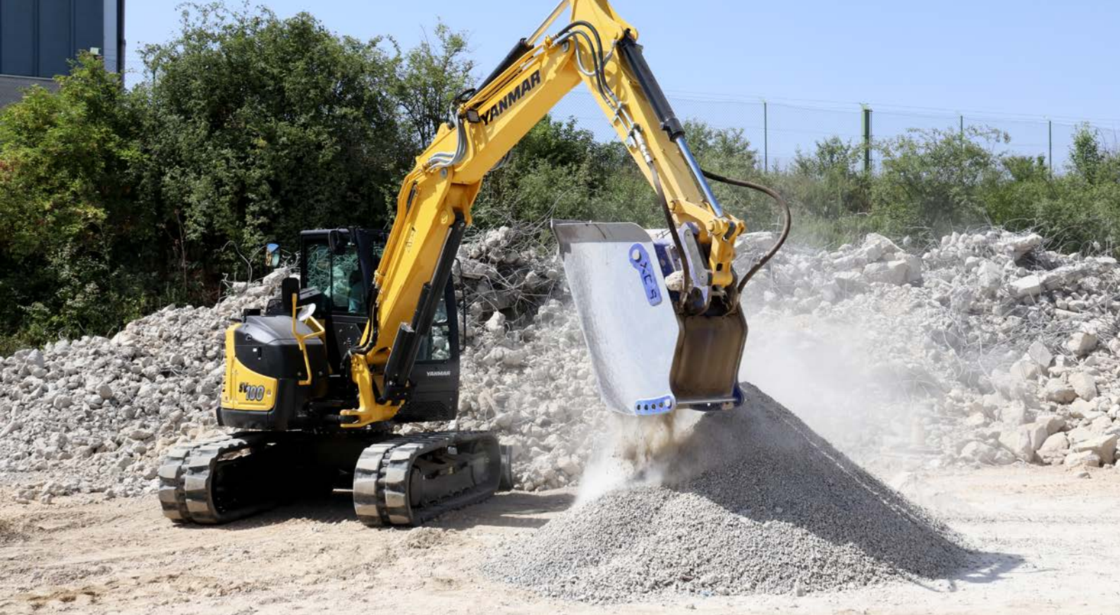
First tests made with the Xcentric Crusher XC9
