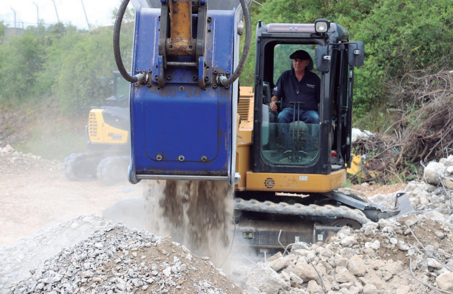
Hervé Prenat testing the first prototype of Xcentric Crusher XC9
