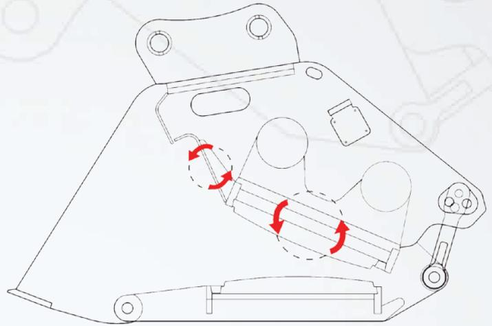
The granulometry adjustment is easy and intuitive, which enables a quick variation.
