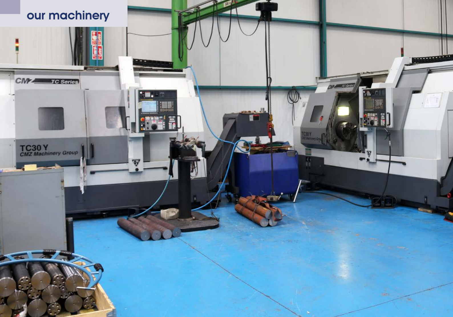
Two CMZ brand lathes, model TC30Y, in the Grado Cero Sistemas machining workshop.
