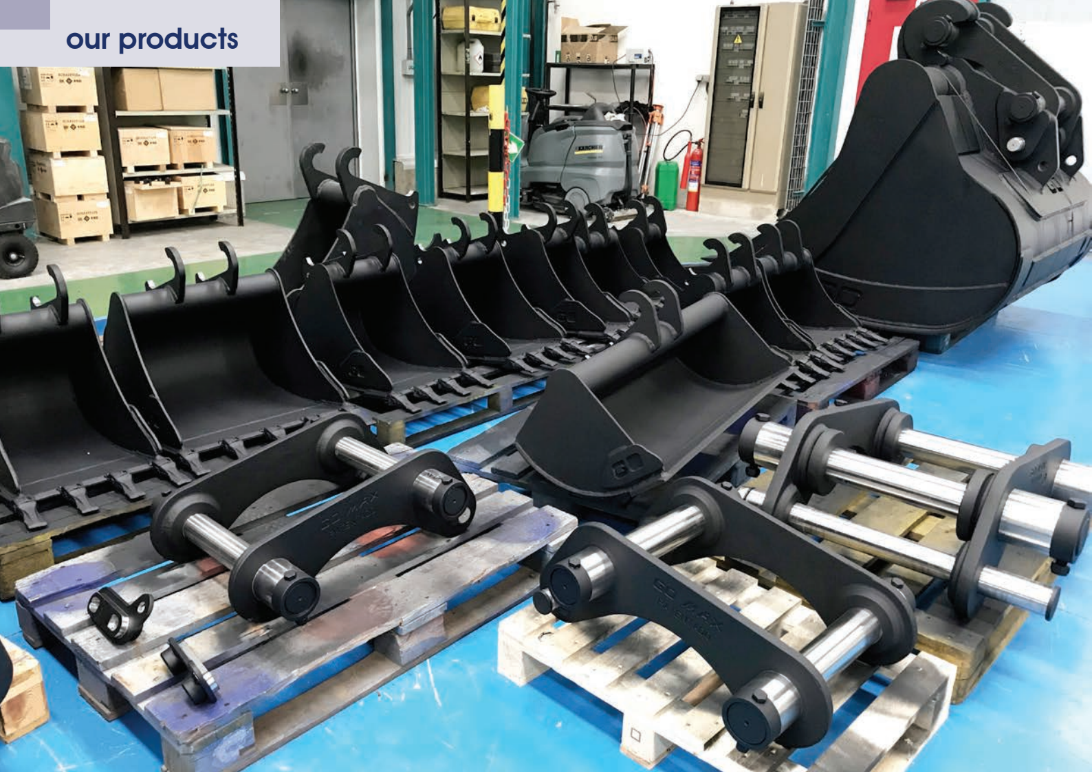
Different finished models of buckets and quick couplers in the workshop.
